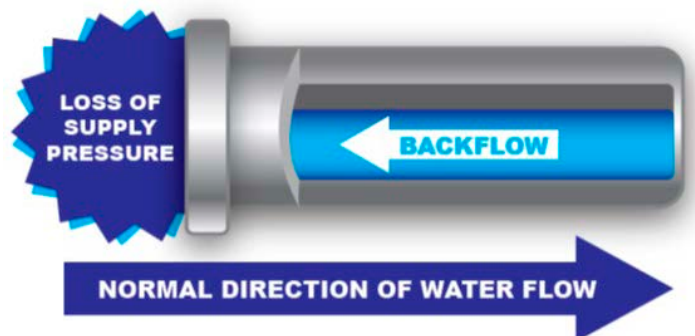
Figure 1: Back Siphonage (Source: City of Durham)
