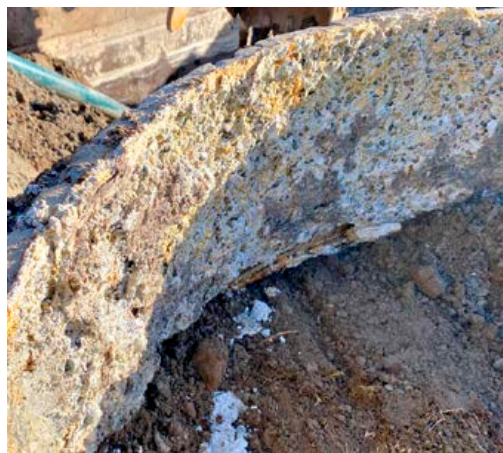
Concrete corroded by Hydrogen Sulphide
