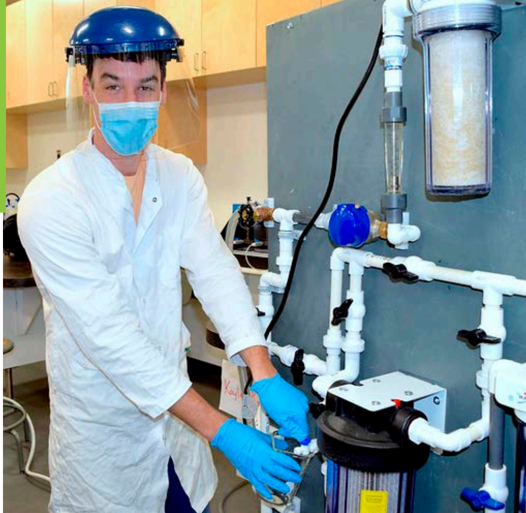
Okanagan College WET Student, Tyler Wilkie, collecting samples to assess the effectiveness of different types of filtration systems
