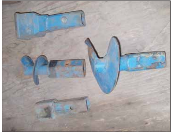
Valve key with various interchangeable fittings
